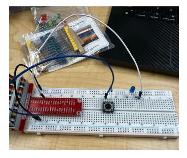
The pull-down resistor is need so that when not pressed the button is at a low state.
